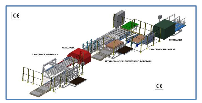
ZAŁADUNEK WIELOPIŁY - loading the multi saw, WIELOPIŁA - multi saw, SZTAPLOWANIE ELEMENTÓW PO ROZKROJU - stacking elements after cutting, ZAŁADUNEK STRUGARKI - loading the planing machine, STRUGARKA - planing machine.
